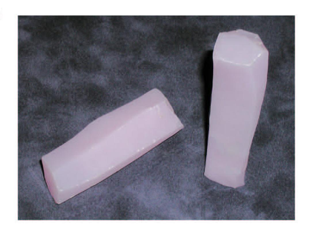
Just like sapphire, the single crystal form of alumina, which has superior properties over ceramic form of alumina, CRYSTAL PSZ has a whole set of improved mechanical properties over the same material fabricated using standard ceramic techniques. For example PSZ crystals have a high strength, (compared to strength of the ceramic form of partially stabilized zirconia) as well as an increased crack resistance.
